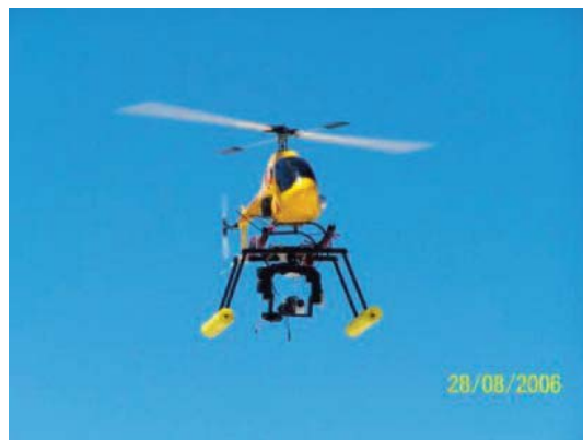
Figure 8. Vellerofontis during a flight carrying a camera streaming video. 87
